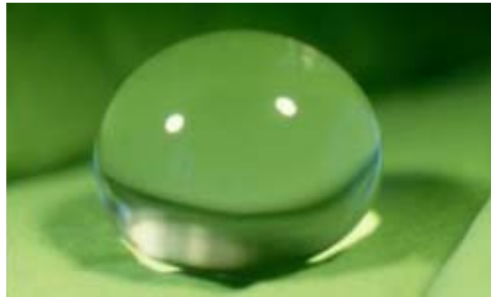
Figure 2. A water droplet on a superhydrophobic surface: the droplet touches the leaf only at a few points and forms a ball. It completely rolls off at the slightest declination (see footnote 6). Reproduced with permission.
